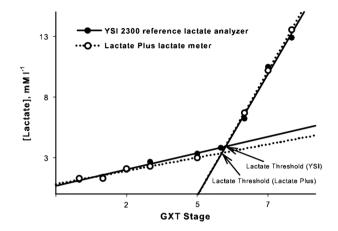
**Figure 1** Determination of the lactate threshold by visual inspection. Shown are data from a representative study participant and the lines of best fit that were determined independently for data from the YSI 2300 lactate analyzer and the Lactate Plus lactate analyzer. Blood samples could not be collected between stages 4 and 5. The Lactate Plus analyzer returned error message between stages 6 and 7.
